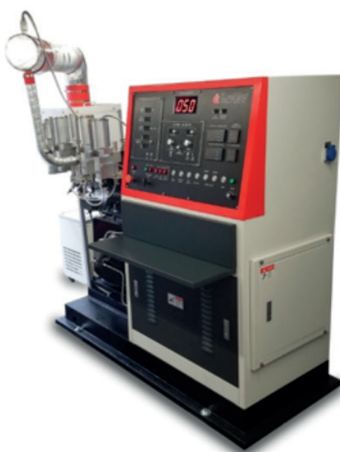
Figure 2: A combination octane rating unit engine octane. This unit (left) is able to determine both MON and RON values. Due to the nature of the device, both tests can be operated using the same chamber. A close-up of the carburetor is shown (right)
