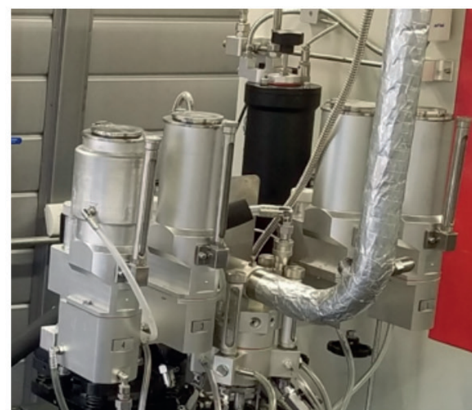
Figure 2: A combination octane rating unit engine octane. This unit (left) is able to determine both MON and RON values. Due to the nature of the device, both tests can be operated using the same chamber. A close-up of the carburetor is shown (right)
