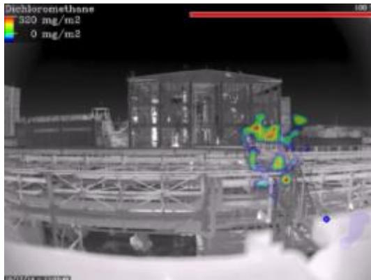
1: The Second Sight® has detected 3 leakages at 100m.
