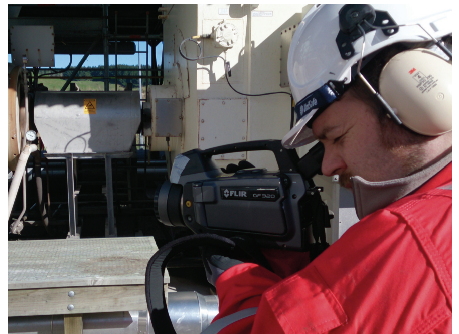
Thanks to thermal imaging cameras, Inspectahire can easily detect gases in difficult to reach or hazardous locations.
