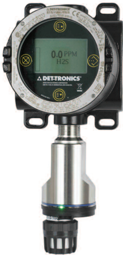
Figure 1: Approved for use in classified hazardous areas, the model UD10 FlexVu® Universal Display is an intelligent field display transmitter that serves as a permanently-connected HART field communicator to HART capable fire and gas detection instruments. It also provides analog/HART, discrete relay, and RS-485 Modbus outputs.
