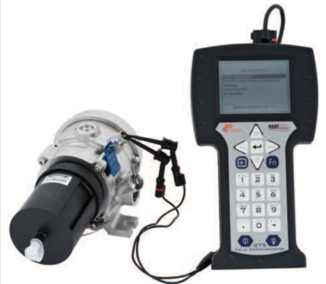
Figure 2: The PointWatch Eclipse® infrared gas detector is available with an optional onboard intrinsically-safe and weatherproof HART communication port, enabling safe and easy field connection to the HART handheld field communicator.
