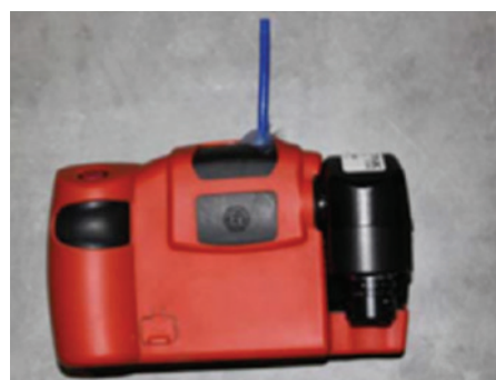
Figure 3 shows the final result of the IP5X testing, after the drop test.
