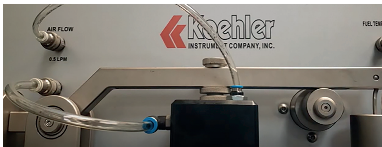
Figure 5. Fully Secured Holder with Lever Arm and Weight
