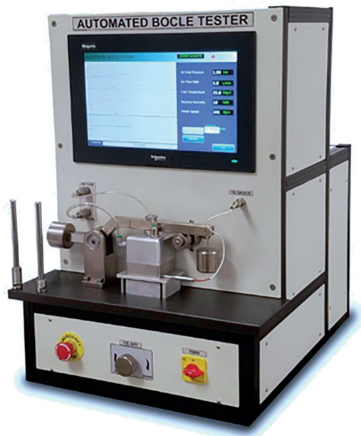
Figure 4. K94100 Automated BOCLE Tester
