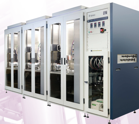
Figure 2: Each Symyx Parallel Fixed Bed Reactor is equipped with 16 individual quartz reactor tubes that enable high throughput, robust experimentation.
