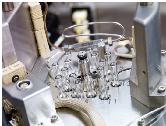
Figure 1: Each Symyx Parallel Fixed Bed Reactor is equipped with 16 individual quartz reactor tubes that enable high throughput, robust experimentation.
