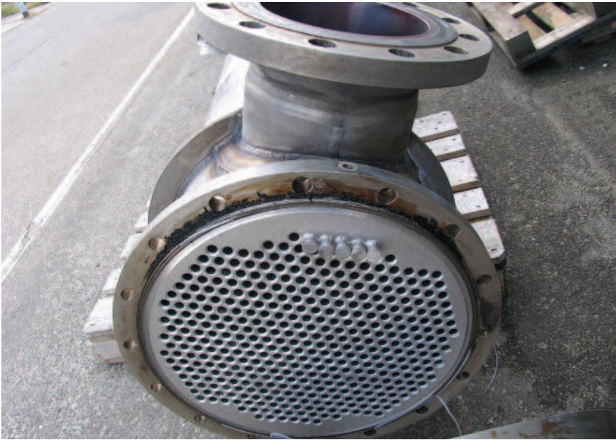
Figure 3: Heat exchanger with 5 plugged heat pipes
