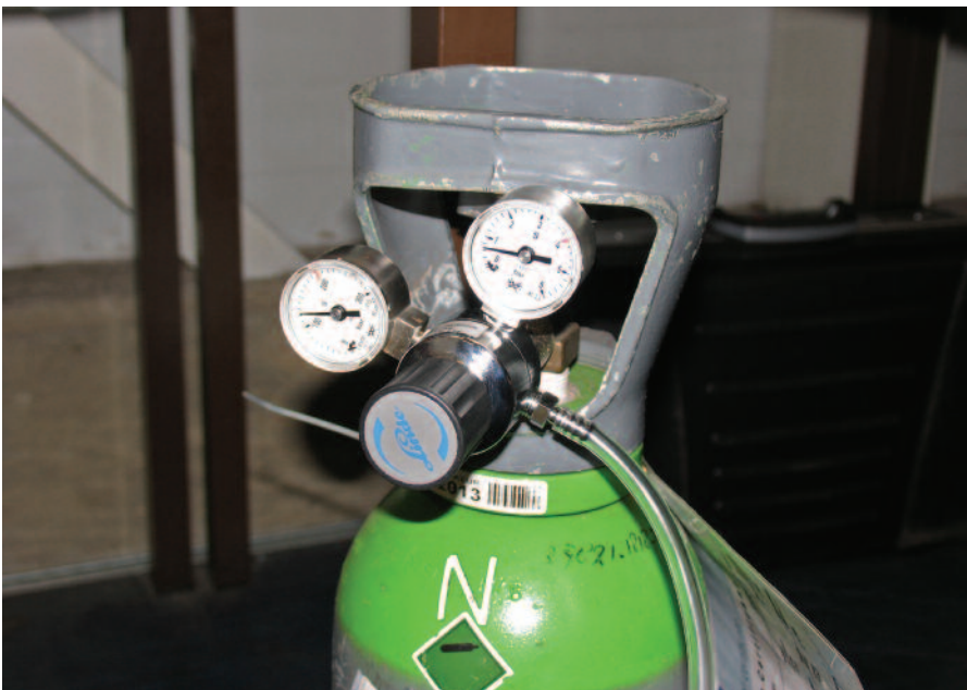
Figure 5: Cylinder with calibration gas
