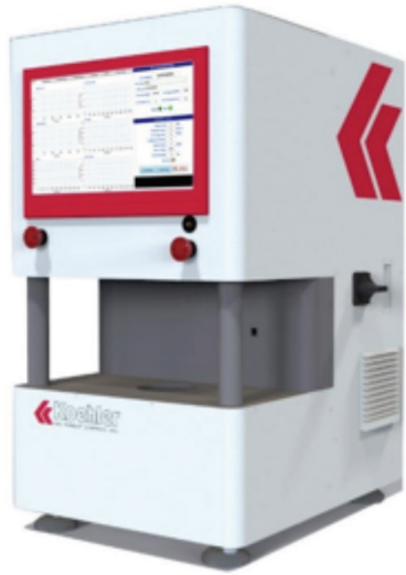
Figure 1: 4-ball wear testing method configuration [8]
