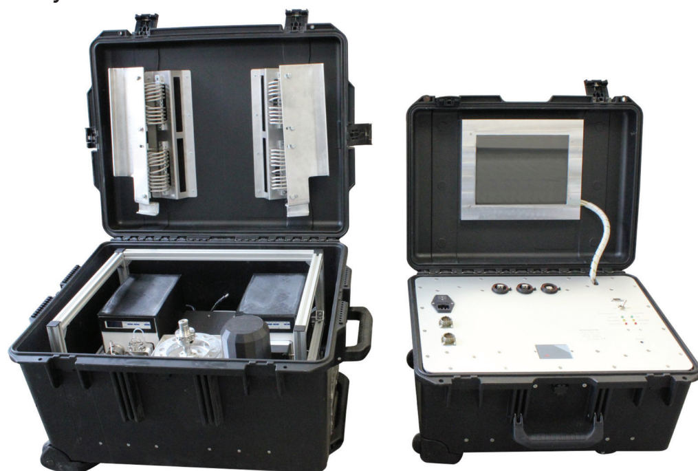
Figure 1: Picture of the transportable GPC-UV: On the left, the analytical module and on the right the module with computer and electronic boards
