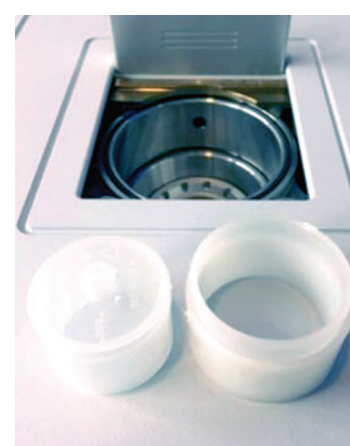
Figure 3: Bruker's dedicated liquid sample cup (Ø 40 mm, left) and the larger SampleCare cup (Ø 51 mm, right)
