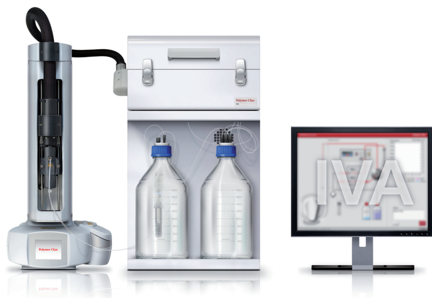
Figure 1. IVA® instrument, fully automated benchtop system for measuring intrinsic viscosity of polymeric materials soluble at room or elevated temperatures up to 200°C, compatible with a variety of solvents. Autosampler including dissolution oven (left), instrument main unit with solvent / waste containers and detectors oven (center) and computer with control and data processing / reporting software (right).
