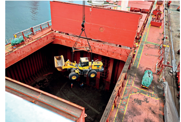
Unloading coal from a bulk carrier
