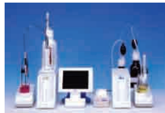
A commercially-available titration system configured for the determination of Water Content, Total Acid Number, & Iodine Value.
