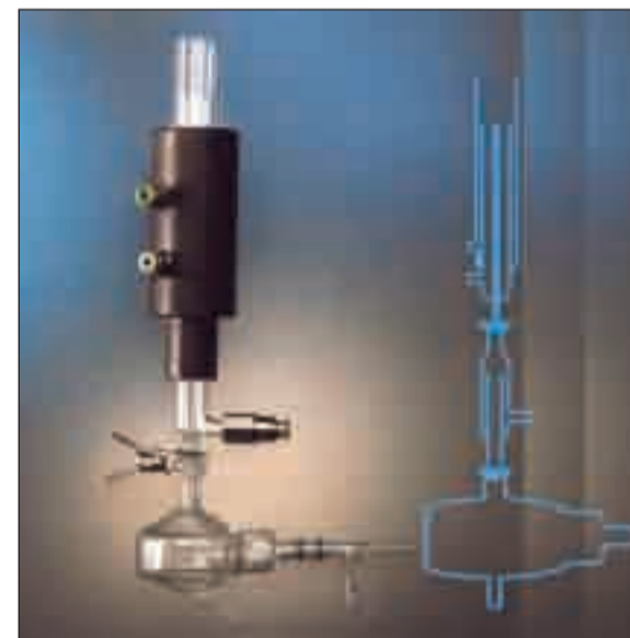
Figure 4: Photograph and schematic drawing of the sheathing gas system
