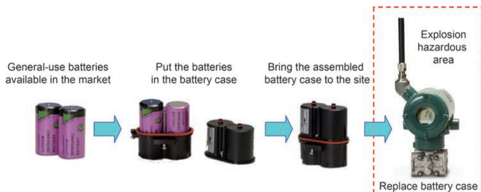
Figure 2: Battery case design allows the use of low cost, commercially available, off-the-shelf, general-purpose lithium thionyl chloride batteries in wireless transmitters. The battery case can easily be replaced, even in a hazardous area environment.
