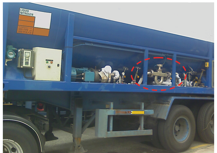
Fig.8: Application example of a Coriolis flowmeter in a road fuel tanker vehicle
