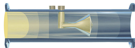
Fig 2. V-Cone Cutaway Showing Irregular Flow Profile
