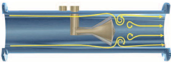
Figure 4: V-Cone Cut-Away Vortices View
