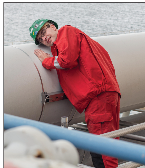
Non-invasive flow measurement by means of ultrasound is obviously an acoustic method.
