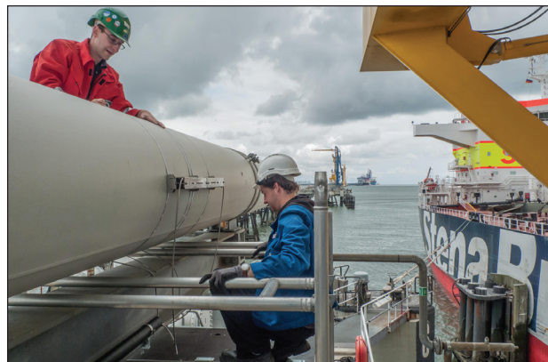
Clamp-on ultrasonic transducers are simply mounted on the outside of the pipeline during ongoing operation.
