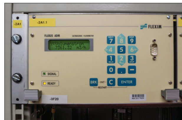
FLUXUS F709 measuring transmitter for installation in the 19” switching cabinet
