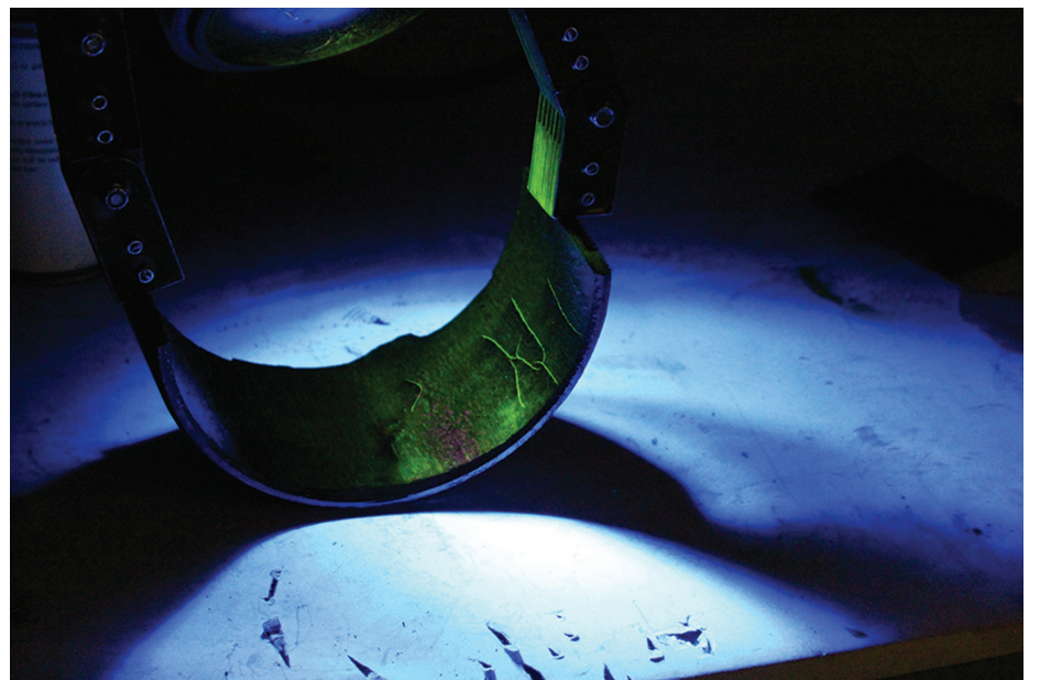
Wet magnetic particle inspection (WMPI) looking for cracks and other manufacturing defects
