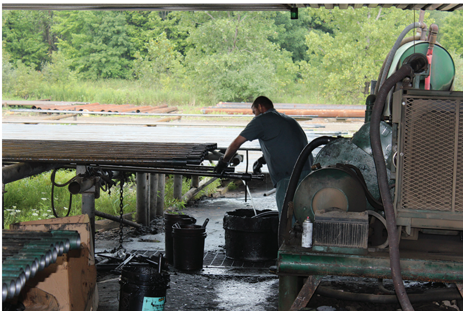
Hydrostatic pressure testing of oil country tubular goods (OCTG)
