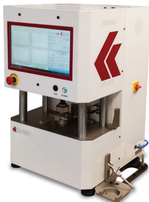
Figure 1: K93170 Koehler Four Ball Wear and EP Tester [5]
