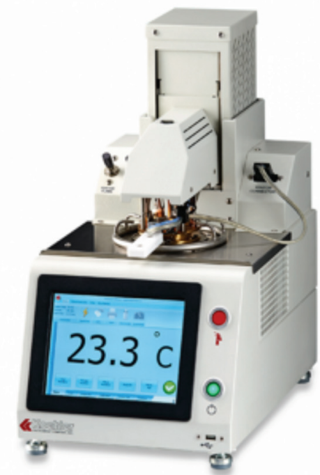
Figure 2. The latest automatic Pensky-Martens Closed Cup Tester (Koehler Instrument Company).
