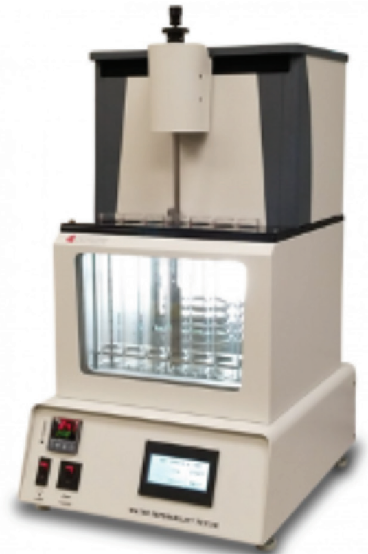
Figure 1 Koehler Water Separability Tester [8].
