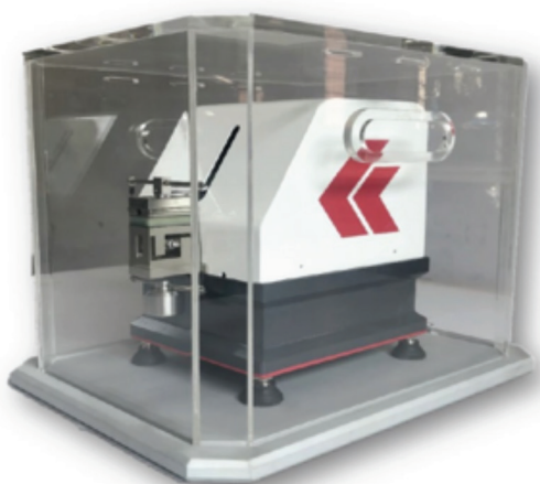
The HFRR instrument (Figure 2) and the ASTM D6079 test method involves rubbing a metal ball in an oscillating motion against a platform metal disk under known conditions while fully immersed in the sample heated to 60 degrees C.
