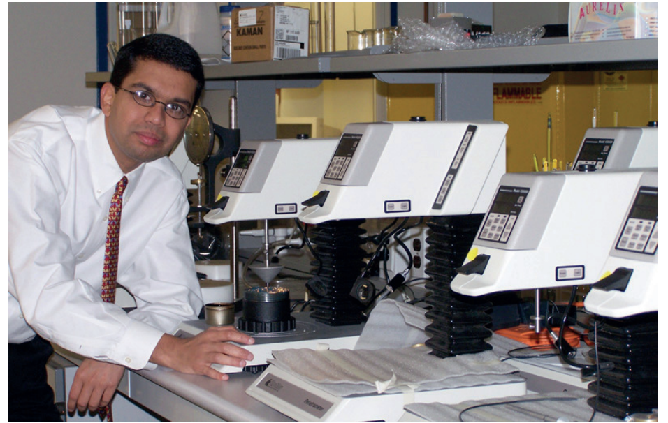
Dr. Raj Shah shown here, at the Koehler instrument company main laboratory in Bohemia, NY working with the new ASTM D217 penetrometer.
