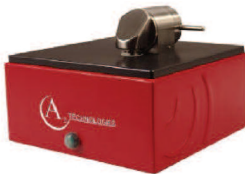
Figure 1: A2 Technologies' PAL FTIR analyzer equipped with TumbIR transmission infrared sampling interface. This system is ideal for table top measurement of % FAME in biodiesel fuel from 0.025% to 20%. The PAL system is 8 pounds and measures 8" x 8". It can be equipped with PDA or computer control.
