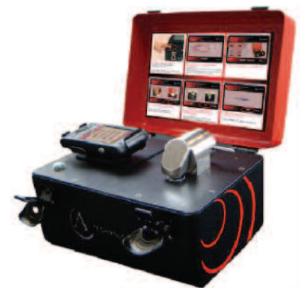
Figure 2: A2 Technologies IPAL FTIR analyzer equipped with TumbIR transmission infrared sampling interface and PDA control. This system is ideal for table top measurement of % FAME in biodiesel fuel from 0.025% to 20%. The iPAL FTIR analyzer weighs 15 pounds and is battery powered for portable use in field applications.
