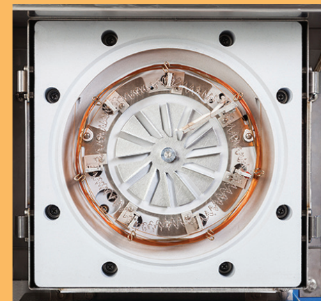
Figure 1: Close up of Wasson-ECE patented Micro-Convection Oven for capillary columns.
