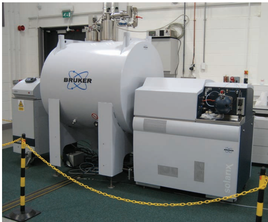
Figure 1: 12 T solariX FTICR mass spectrometer located in the Ion Cyclotron Resonance Laboratory (University of Warwick, Coventry, UK).
