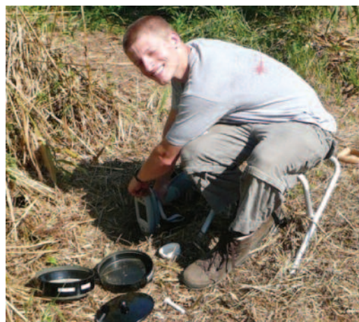
Figure 5. Soil analysis by handheld EDXRF instrumentation (according to the EPA Method 6200)
