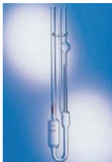
Figure 1: Viscometer manufactured by Thomas Scientific (Thomas Scientific, 2013).
