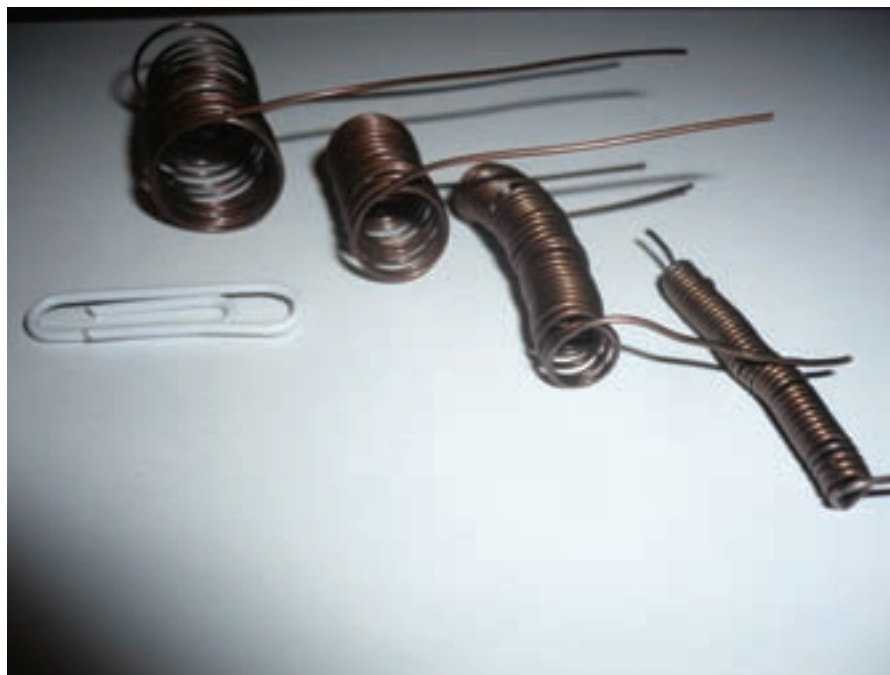
Figure 1: Micropacked columns from Restek can be coiled to fit any GC.
