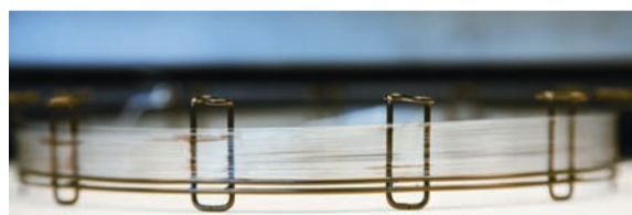
Figure 1: MXT®-1HT Sim Dist columns are unaffected by high method temperatures. In contrast, the coating on fused silica columns can be damaged and may delaminate completely, significantly reducing column lifetime. (Fused silica column, 72 hours at 430°C).
