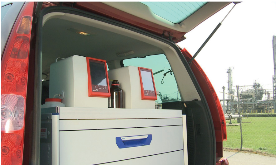
Figure 3: ERACHECK – a portable and rugged oil-in-water analyzer
