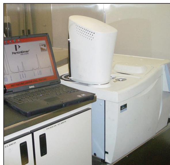
Figure 4: PerkinElmer's Clarus GC System used to test IndyCar fuel (Courtesy of PerkinElmer Inc.)
