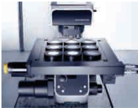
Figure 2: SGS uses a special multi-filter holder insert which can have up to 9 filters mounted on it simultaneously. The analysis is then conducted and evaluated automatically providing considerable time savings compared with filter analysis using just one filter holder.
