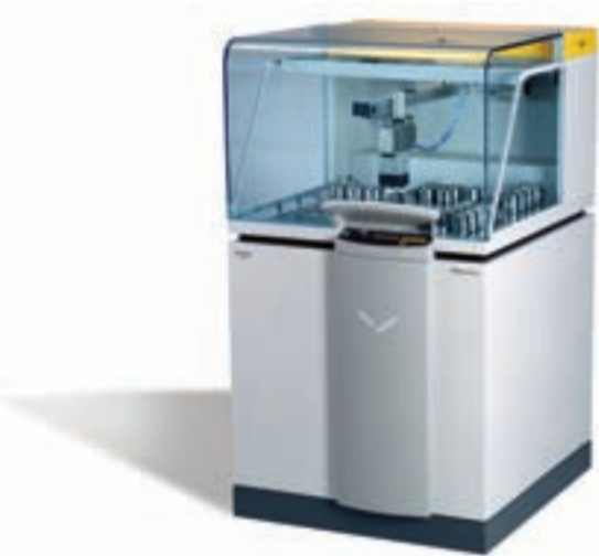
Figure 1: PANalytical's Axios-Petro wavelength dispersive X-ray fluorescence spectrometer
