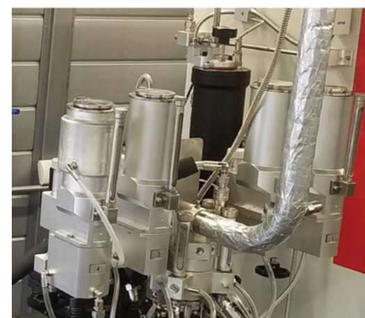
Figure 1: Combination Octane Rating Unit Engine produced by Koehler Instrument Company.
