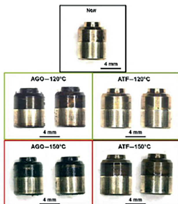
Figure 6: Brass Bearings at the end of the Solenoid test [7]
