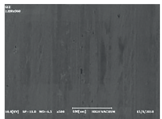
Surface Y - the desktop scanning electron microscope representation of the surface corresponding to the 1% wt nano grease test. Reprinted from [13]
