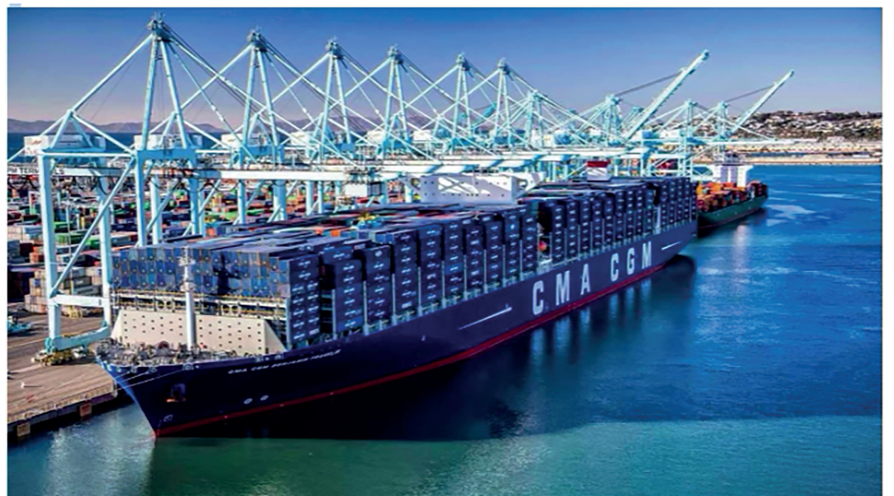
Figure 1: The CMA CGM Benjamin Franklin, one of the largest cargo ships to ever visit the U.S. An ultra-large container ship measuring 399.2 m in length, 54 m in width, and 60 m in height. The vessel carries 4.5 million gallons of fuel oil and consumes 330 tons of fuel daily 2 .
