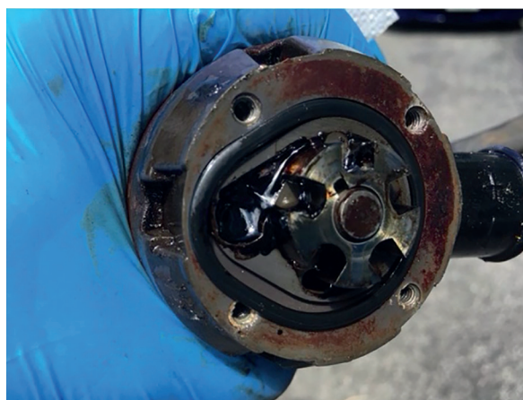
Figure 2. Gummed up fuel pump from a car [7].
