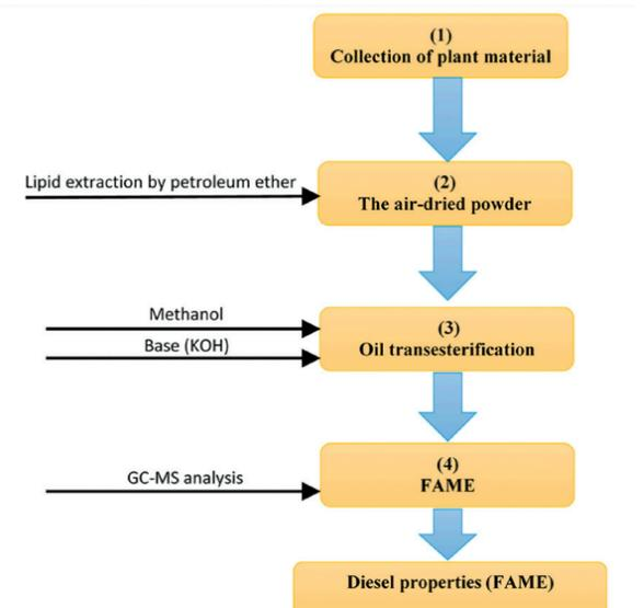
Figure 8. Stepwise process of FAME production [4]
