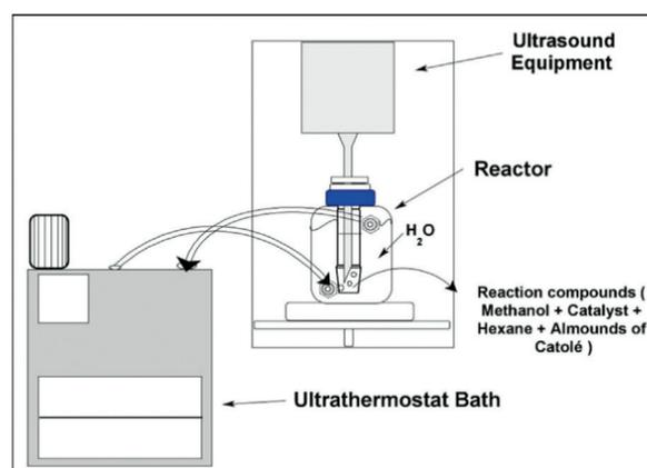
Figure 2. Reactor diagram showing the emulsification process [1]
