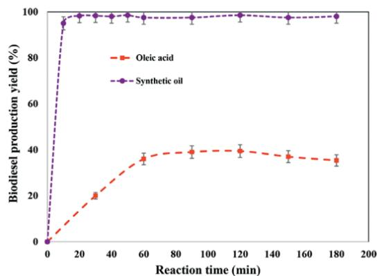
Figure 11. Correlation of reaction time with biodiesel yield [7]
