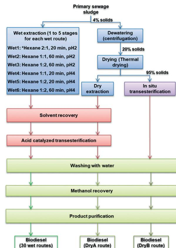
Figure 15. Flow chart showcasing various biodiesel production methods using sludge [9]
