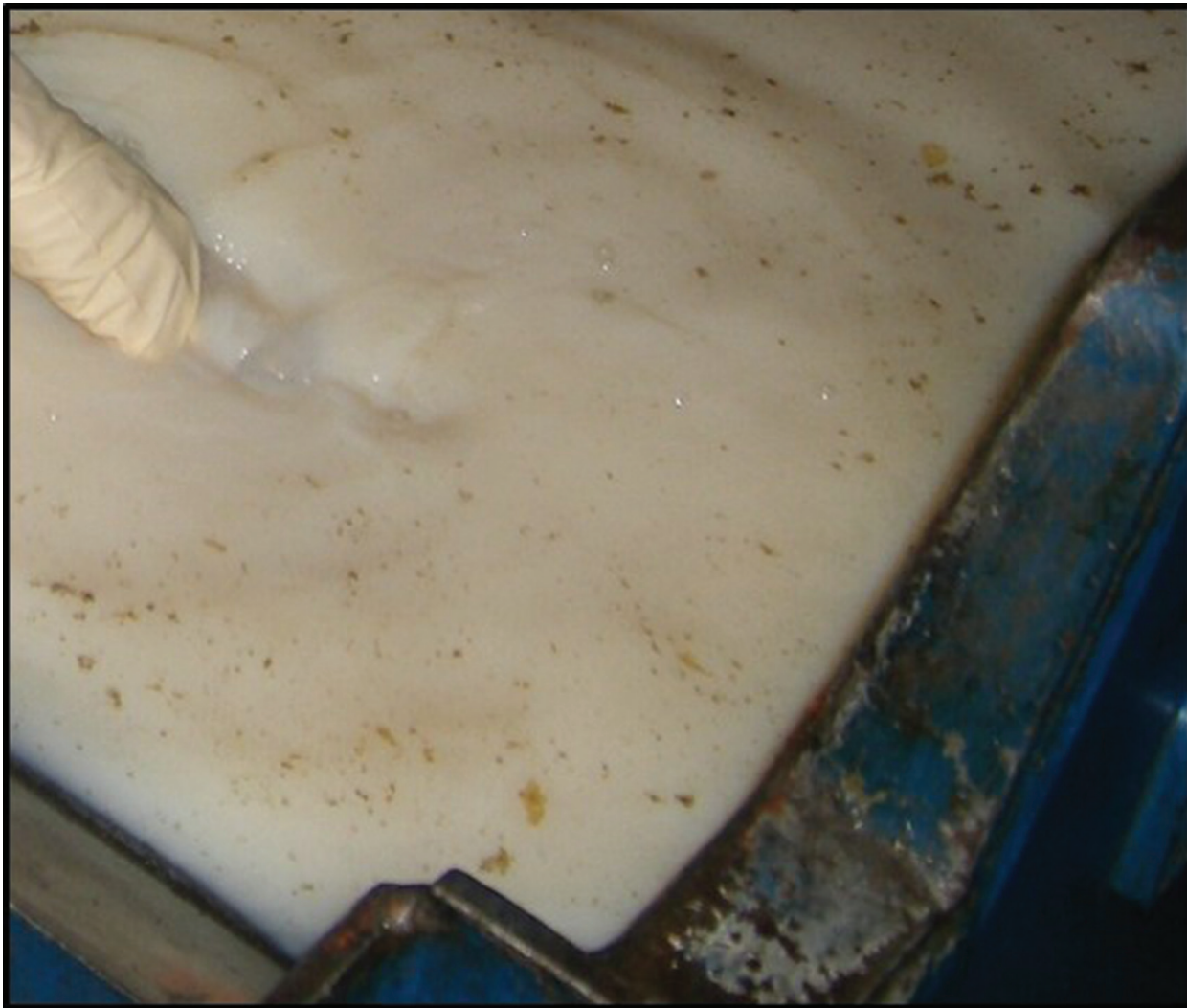
Collecting a grab sample of emulsifiable oil MWF from an individual machine sump.
