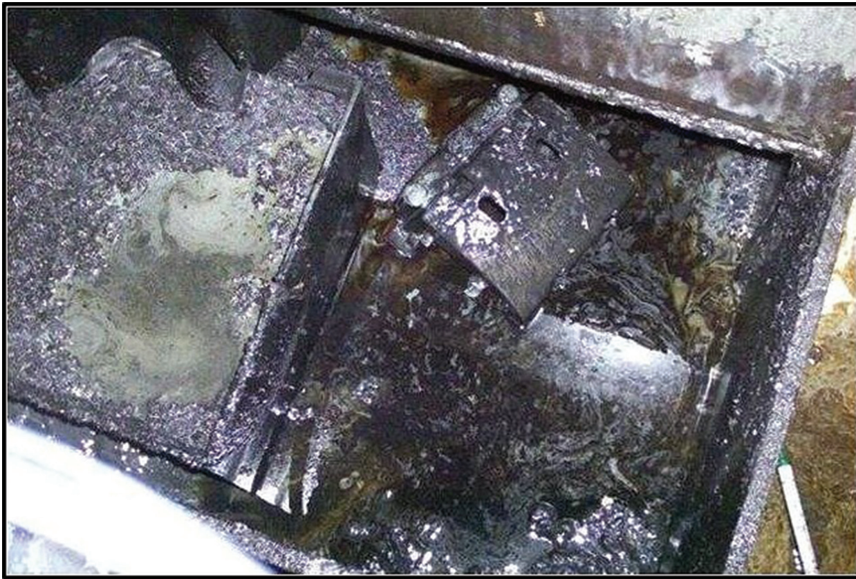
Individual machine sump - example of bad practice. If the system is not kept clean, the best MWF will fail.
