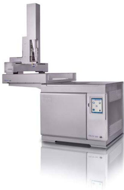
Figure 1: Master GC Fast Gas Chromatograph equipped with MASTER AS Liquid Autosampler
