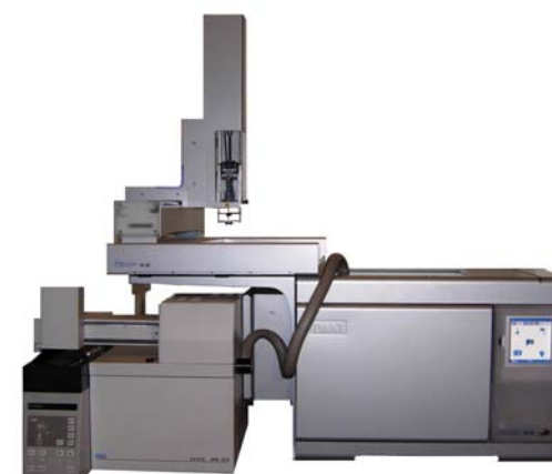
Figure 5: Master GC unit combined with the Master AS Liquid Autosampler is easily hyphenated to the HSS 86.50 Head Space Sampler
