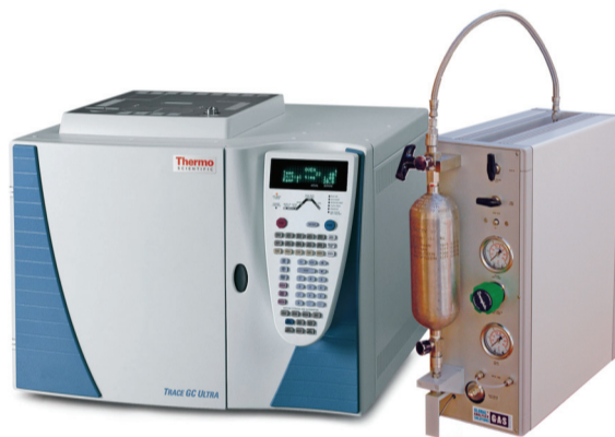
Figure 2: LPG analyser with LSV and Pressure Facility, which is available for different sample cylinder sizes and connectors.
