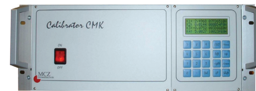
Figure 12: Calibrator module for generating/diluting calibration gases.
