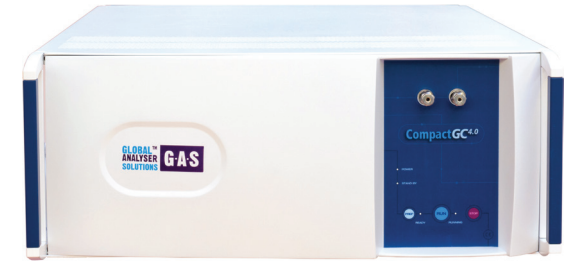
Figure 10: CompactGC 4.0 : 19" analyser with thermal desorption module and PFPD.
