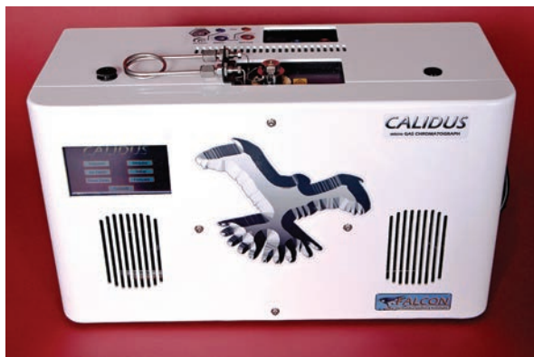
The Calidus Gas Chromatograph cycles 10 to 50 times faster than traditional GCs.
