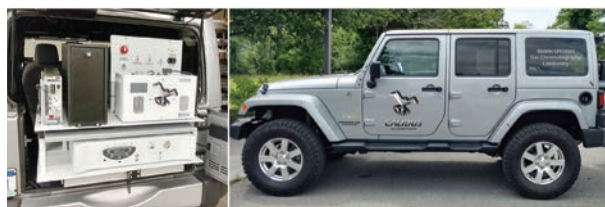
A Calidus GC Mobile GC System like the one used for HMRC fuel fraud detection.
