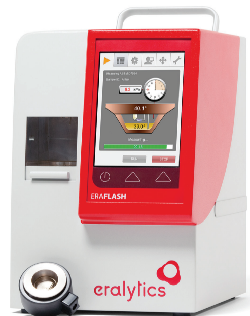
Figure 5: ERAFLASH analyser with the 2ml sample cup for ASTM D7094 compliant measurements
